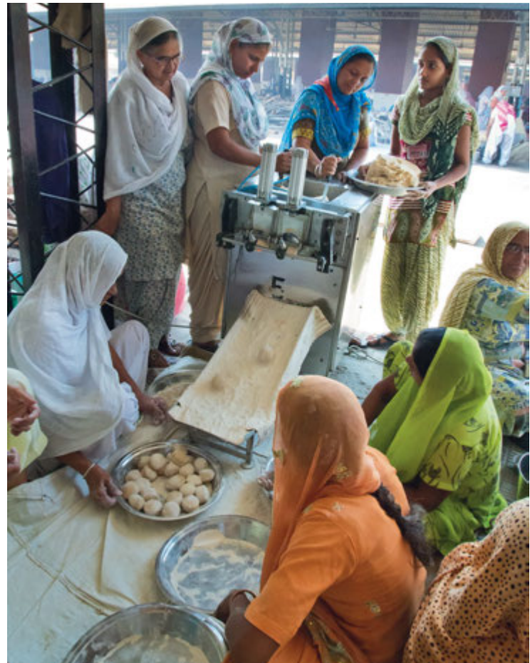
A peda (dough ball) making machine is used to make small individual-size dough balls. This greatly speeds up the chapati-making process and ensures that each chapati will be of a uniform size.
