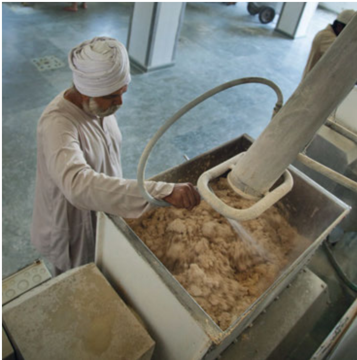
A peda (dough ball) making machine is used to make small individual-size dough balls. This greatly speeds up the chapati-making process and ensures that each chapati will be of a uniform size.
